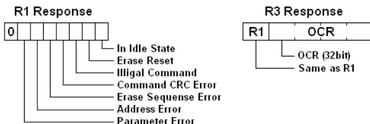
There are some command response formats, R1, R2, R3 and R7, depends on the command index. A byte of response, R1, is returned for most commands. The bit field of the R1 response is shown in right image, the value 0x00 means successful. When any error occurred, corresponding status bit in the response will be set. The R3/R7 response (R1 + trailing 32-bit data) is for only CMD58 and CMD8.
